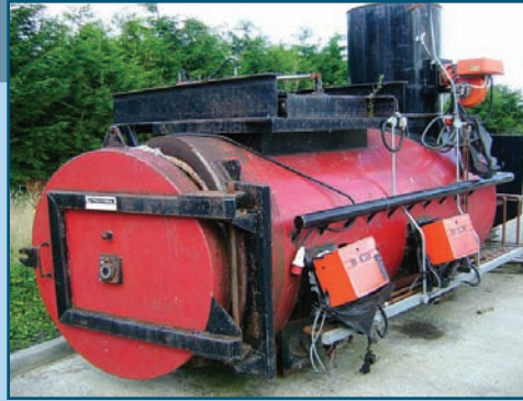
Techtrol Pyrotec A50L semi automatic top loaded carcass incinerator
